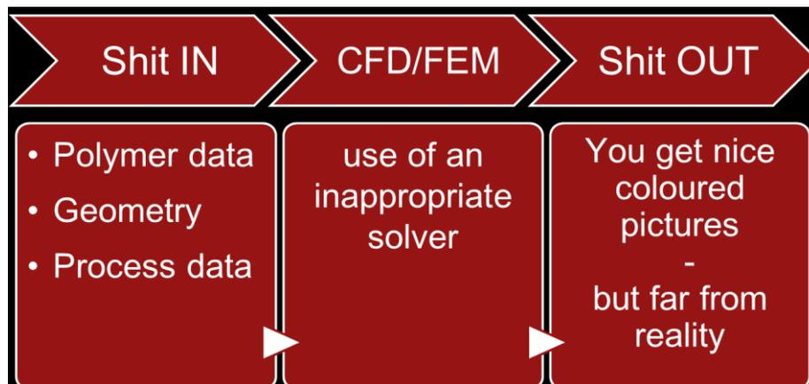
If the used polymer data do not correspond to those of the processed material, the simulation cannot represent the real process. In addition, of course, you should note that solvers for turbulent air flows are completely unsuitable for studying laminar polymer flows. You will always get colorful nice pictures. The accuracy of the results of a simulation depends mainly on the used solver and the correspondence of the entered boundary conditions with the actual conditions.
