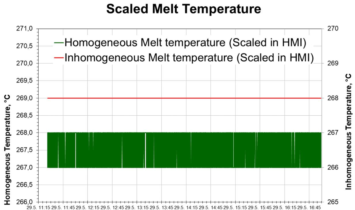
As the melt temperature can only be measured during production with the sensor technology available in the line, this parameter is of great importance. It should be noted that the measured value is strongly dependent on the type of sensor and the installation situation. In absolute terms, therefore, the value cannot reflect the actual temperature - but this does not affect the constancy!
